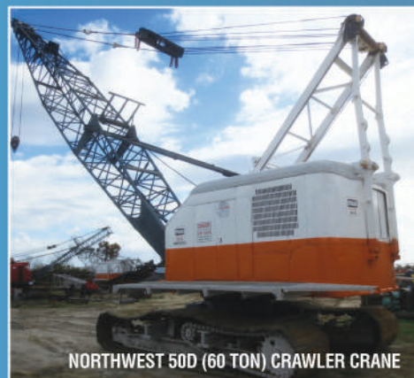
NORTHWEST 50D (60 TON) CRAWLER CRANE
